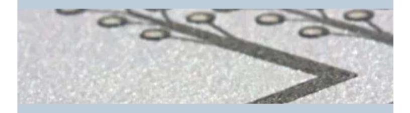
LOCTITE ECI 1501 E&C is a formable, conductive silver ink with a good elongation performance. It is often used to print formable circuits to create 2.5 to 3D shaped circuits and in-molded electronic (IME) solutions. LOCTITE ECI 1501 E&C has a possible elongation to break of ±50%. It is suitable for screen printing and compatible with polyester, polycarbonate, and some TPU foils.
