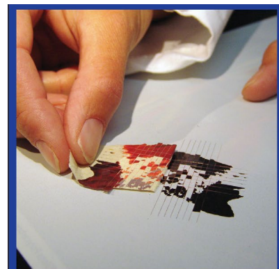
UV Injet printed uncoated polycarbonate fails the ASTM D3359 tape test.
