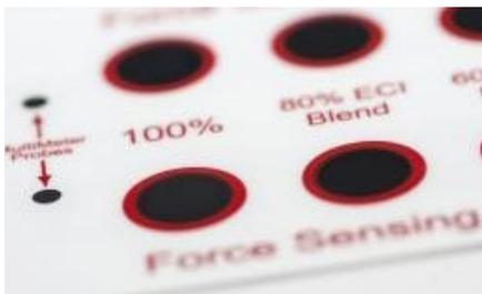
E&C to adjust resistance levels in the range of 50 till 500,000 ohms/sq/25µm. Targeted force sensing applications are wide reaching, from: medical, consumer electronics, musical, commercial and industrial end uses.
