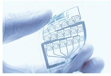
in the printed electronics industry where silver ions move between two printed silver traces with voltage potential, usually when there is an electrolyte such as moisture present within the circuit. This will cause the circuit to short. However, if constructed effectively, coating silver traces with inert dielectric inks can significantly reduce the chance of silver ions migrating even in the presence of moisture.
