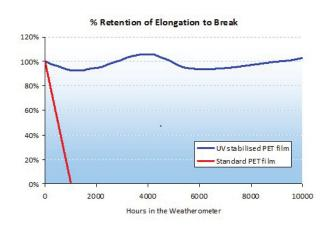
This lifetime enhancement can be offered as a clear film (light transmission up to 94%) or in hazy or opaque films. It can also be combined with a wide array of pretreatments for handling and adhesion of inks, coatings, or other laminate layers, as well as, enhanced thermal stabilization (e.g. 30 minutes at 150C).
