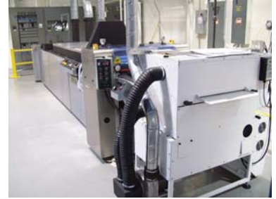
Tekra's newest equipment investment: A high speed sheet coater for small runs of custom materials.
