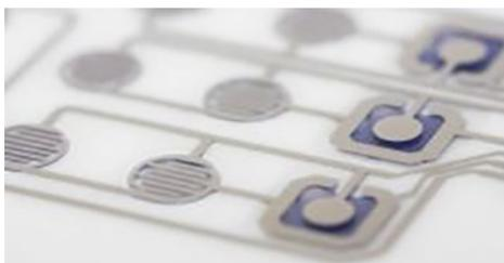
Loctite® ECI 1010 E&C and ECI 1011 are the newest silver ink compositions available from Tekra, A Division of EIS, Inc. Both products allow for improved design flexibility, increased conductivity, and permit the deposition of thinner lines and thinner print thickness – resulting in material savings.
