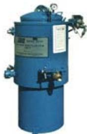
To be installed in Q4 of 2010, the solvent recovery system distills and cleans the dirty solvents left over after cleaning. Through a combination of heating and cooling, the contaminants and solvents can be separated and recovered. After running through a cycle, the dirty cleaning solvent is now free of contaminants and can be used again and again. The remaining solids, instead of being hazardous waste, now can be added to Tekra's polymer recycling stream.
